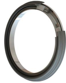
The LEVITEX seal is a cost-optimized, dry gas seal, which can be assembled on a combustion engine crankshaft in place of a conventional oil seal. This concept of dry gas sealing is already in mass production in many different applications, e.g., steam turbines, turbo chargers, and compressors.
